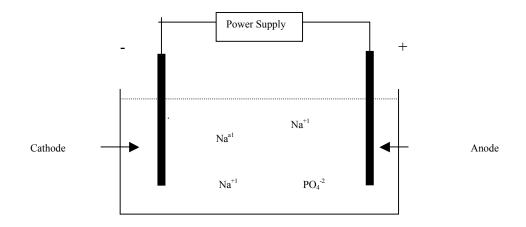
A stainless steel cathode is used in the cell. Water is reduced at the cathode.
